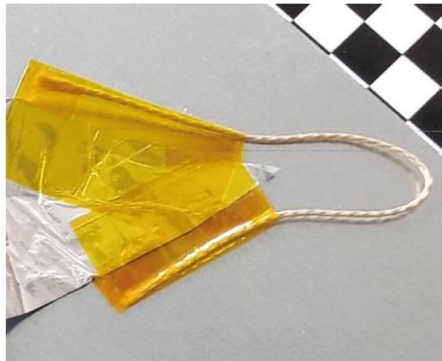
**Fig. 8. Kevlar loop allows for fine adjustments when tensioning sail.**
