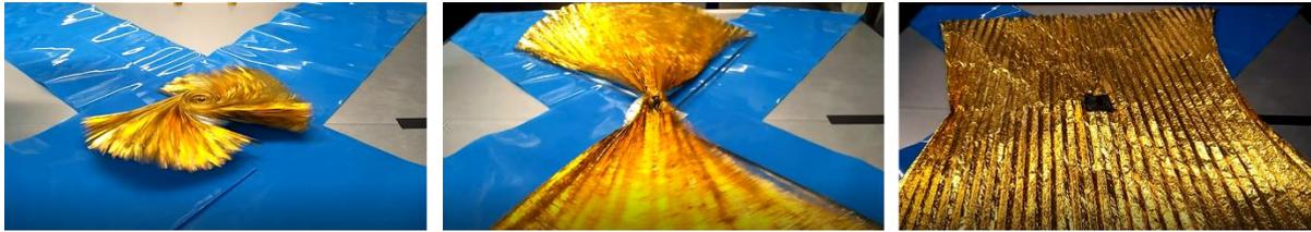
**Fig. 9. Deployment tests carried out on table with low-friction polymer tracks.**
