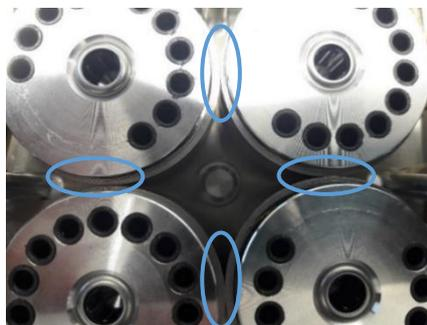
**Fig. 5. Radial blooming and rotational instability lead to rubbing and prevent complete deployment**
