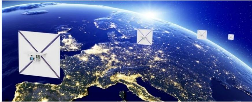
**Fig. 1. Artist impression of ERNST 12U CubeSat with planar drag sail de-orbit system**
