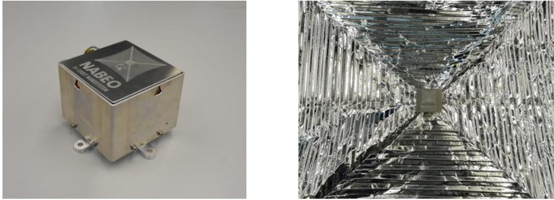
**Fig. 11. NABEO in stored and deployed configurations.**
