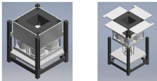
**Fig. 2. First stage of deployment: telescopic motion out of 1U housing [4]**
