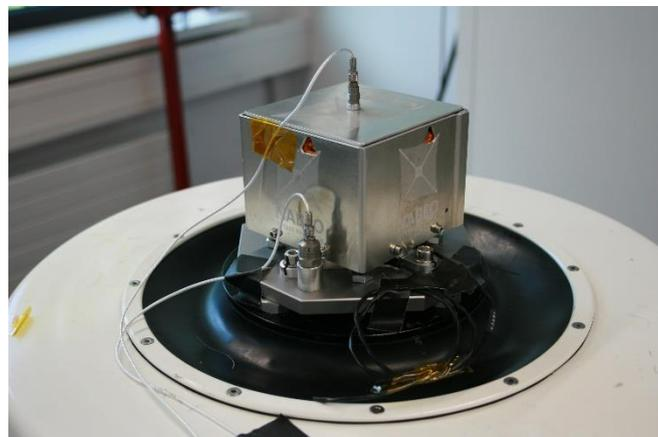
**Fig. 10. NABEO mounted to vibration test platform at Fraunhofer EMI**
