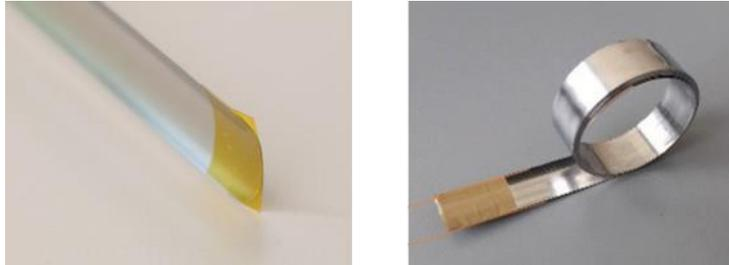
**Fig. 3. Stainless steel tape spring booms are bi-stable, in rolled and unrolled configurations**
