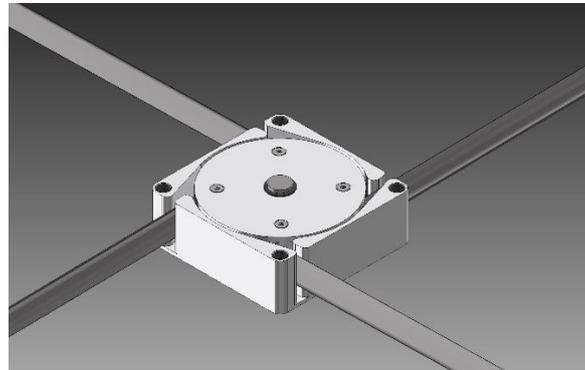
**Fig. 6. Transition to single boom-spool to reduce number of moving parts and prevent boom interactions**
