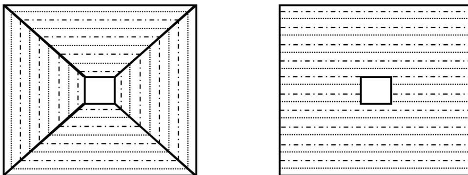
**Fig. 7. Two folding pattern options for single piece sail; dashed lines represent mountain-valley folds.**
