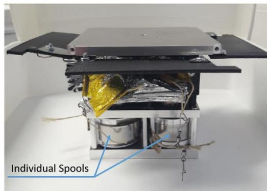
**Fig. 4. EDOS breadboard prototype with four boom spools and sail cartridges [4]**
